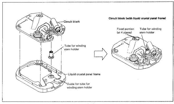
The circuit block of Cal. L823 is heat-combined at 4 places with the liquid crystal panel frame after setting the tube for winding stem holder in the liquid crystal panel frame and placing the circuit block on it.
