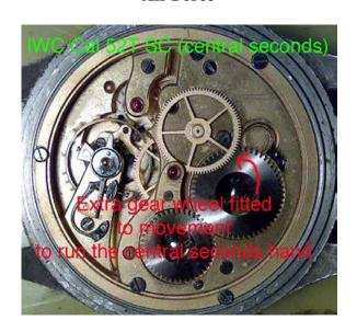
For the IWC enthusiast and collector you may wish to know that the IWC factory ledger list the diameter as not as 19 lignes but 19/22. The '22 lignes' appears because the movement was outfitted with a movement ring that increased the diameter to 22 lignes for fitment into the large case.
