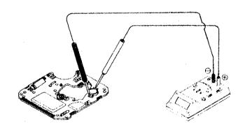
(3) Check the appearance of piezoelectric element.
