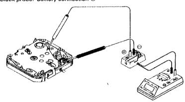
2. If the current consumption is more than 3.0  $\mu$ A, check the current consumption for the circuit block alone.
