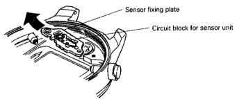
9 Circuit block for sensor unit
