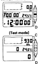
2. Open the case back and turn the trimmer resistance for pressure adjustment (Trimmer A) to set the atmospheric pressure within to  $\pm 2$  hPa of the actual atmospheric pressure.
