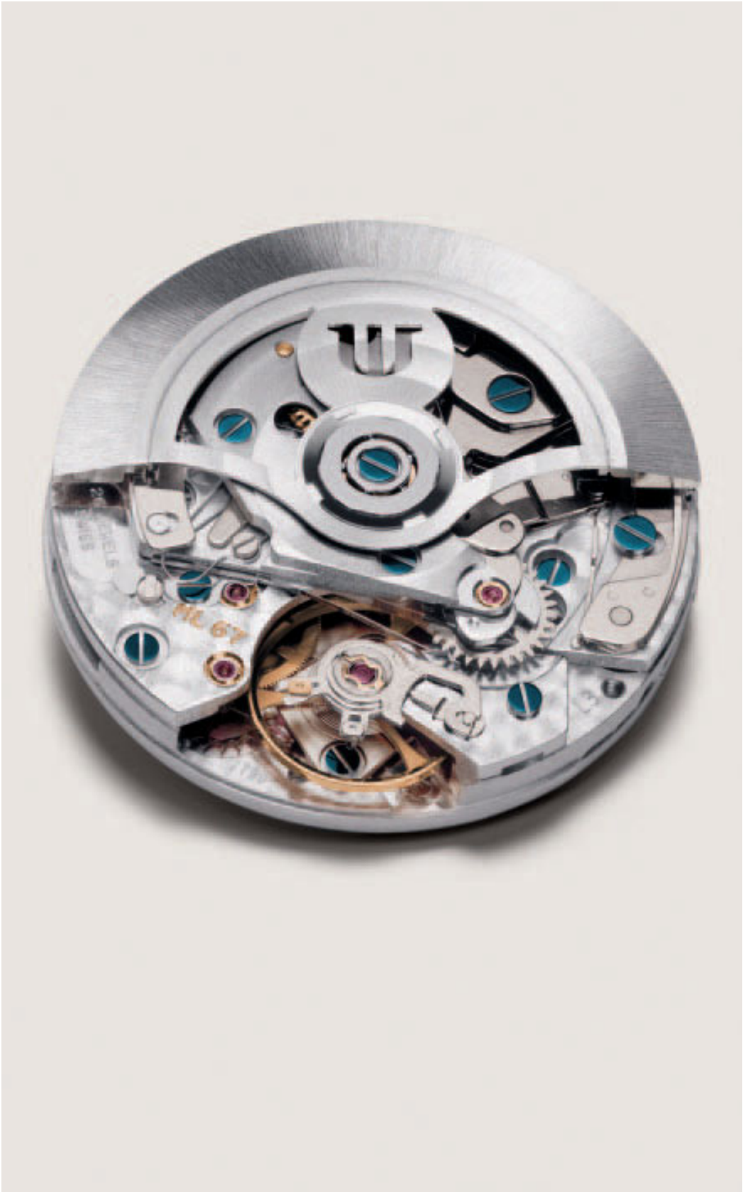
The ML 67 calibre. The automatic Valjoux 7750 chronograph has a stop function with \frac{1}{8} second precision, 30-minute and 12-hour counter, as well as weekday and date indication. However, an intricately decorated surface, blued screw heads, 26 jewels, a first-rate oscillation and escapement system, as well as a five-position adjustment distinguish this finished movement of the Croneo from the basic movement.
