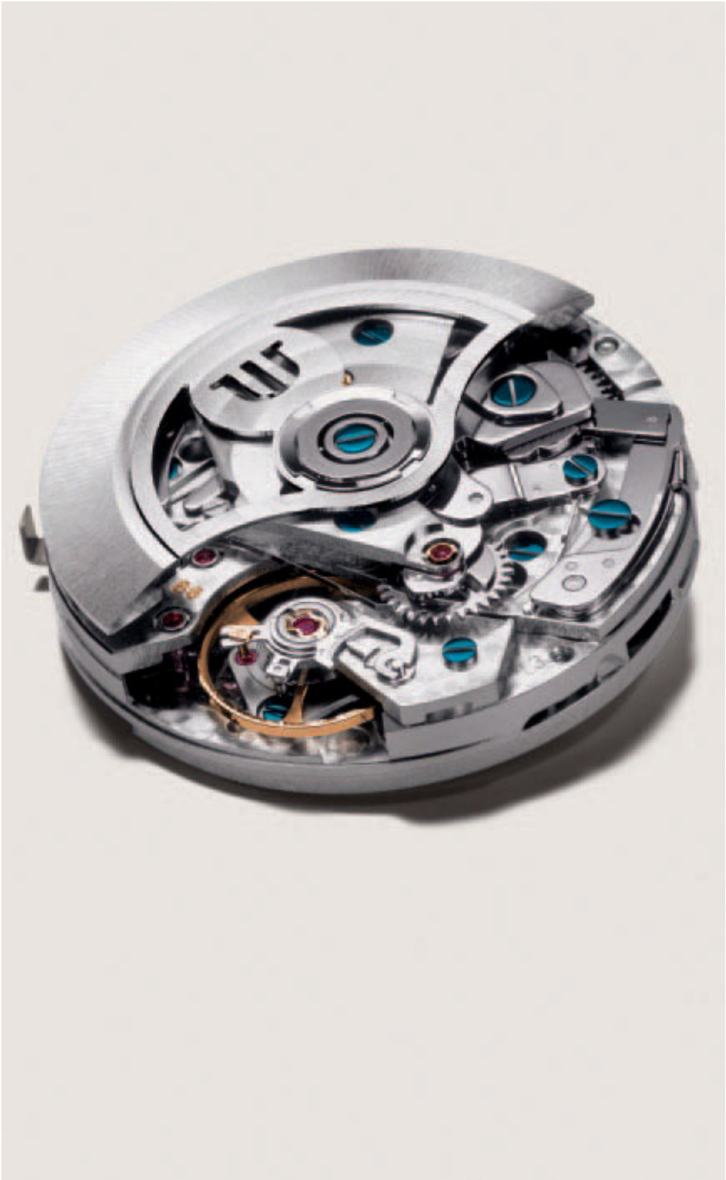
The ML 88 calibre. As a result of its skeleton rotor, this automatic chronograph movement is presented openly. In addition to hours, minutes, seconds, and date, two additional time zones are displayed.
