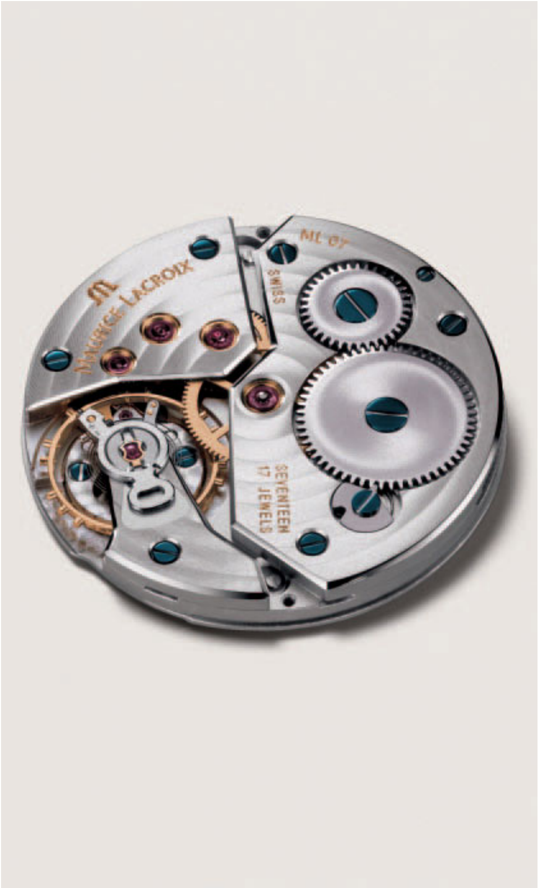
The ML 07 calibre. The inner working of the Jour et Nuit is characterised by the highest level of craftsmanship: It consists of a rhodanised, perfectly crafted and finely decorated ML 07 calibre, based on the Uitas 6498-1 pocket watch movement.
