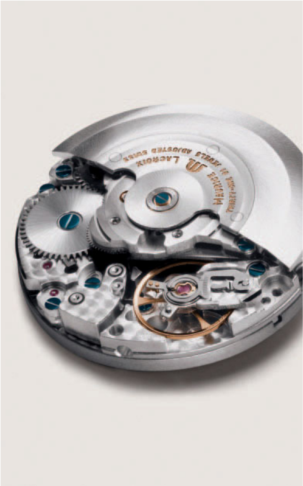
The ML 06 calibre. The automatic alarm movement is based on the legendary AS 5008 calibre. It was meticulously optimised for Maurice Lacroix, equipped with ball bearing rotor and 31 jewels and lovingly hand-decorated and finished, reflecting the highest level of watch-making art. Two barrels – one for the watch movement, the other for the alarm – ensure that an activation of the alarm function does not affect the watch movement power reserve.
