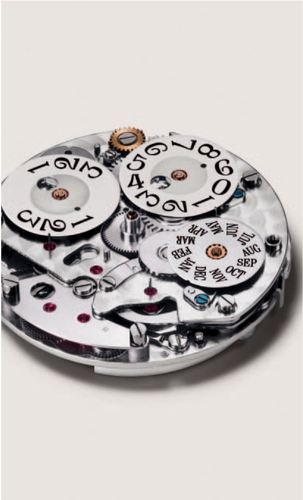
The ML 15 calibre. Three disks for indication of date (first and second digits) as well as month.
