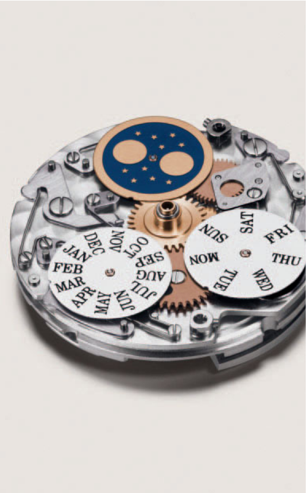
The ML 37 calibre. It is this complicated heart of the Phase de Lune together with the balanced design that makes this Masterpiece so attractive: A complex train of wheels controls the weekday, month, and moon phase displays via three separate disks.
