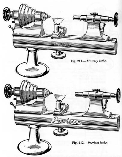
Peerless. Similar to the Marshall and Moseley lathes, with cone bearings. A little lower priced (Fig. 212).
