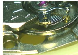
4. Using sturdy tweezers, set the stud to the stud support and press it down.
