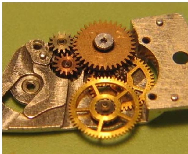
Dual reverser wheel system of the Longines 430/1/2/3 series. Photo: courtesy Jim Hodek
