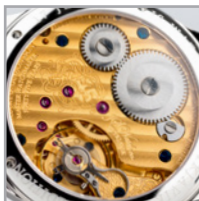
Modified and decorated Unitas movement.
