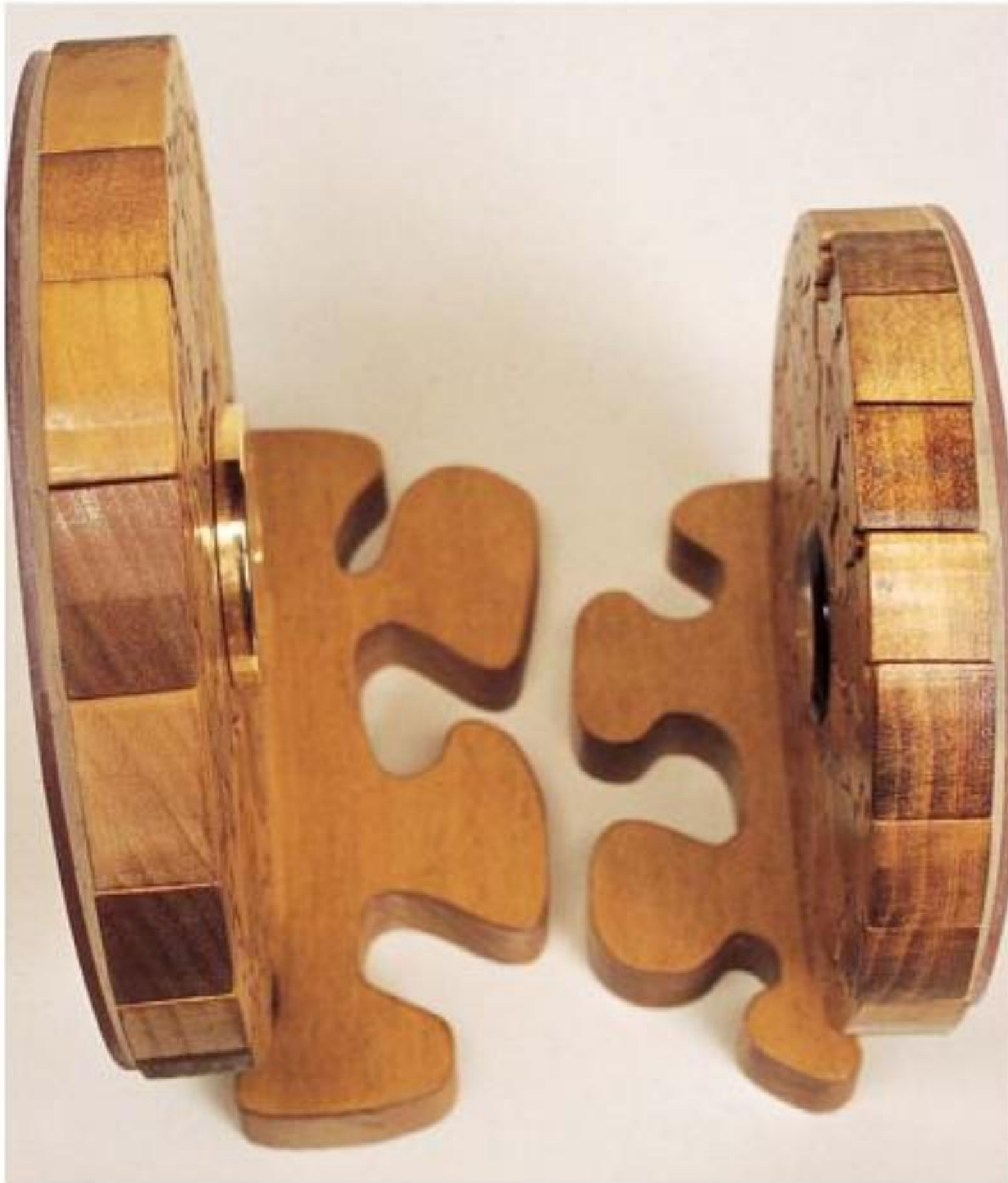
Home base: The bases of these clocks were shaped in classic puzzle piece form. Glue the bottom piece of the face of the clock to the base. The backing board is attached to the base via two round head \frac{1}{2} " wood screws.
