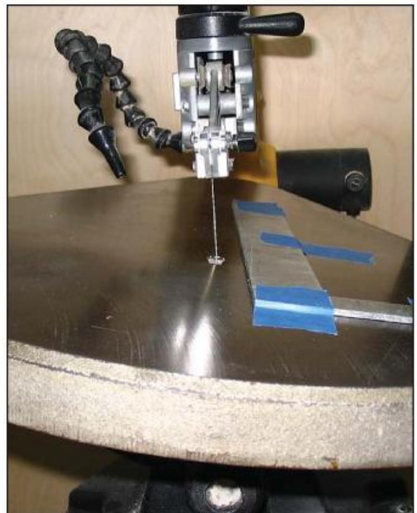
Always check that the table is 90° relative to the blade. This table and blade obviously don't form a 90° angle, but some differences won't be as obvious.
