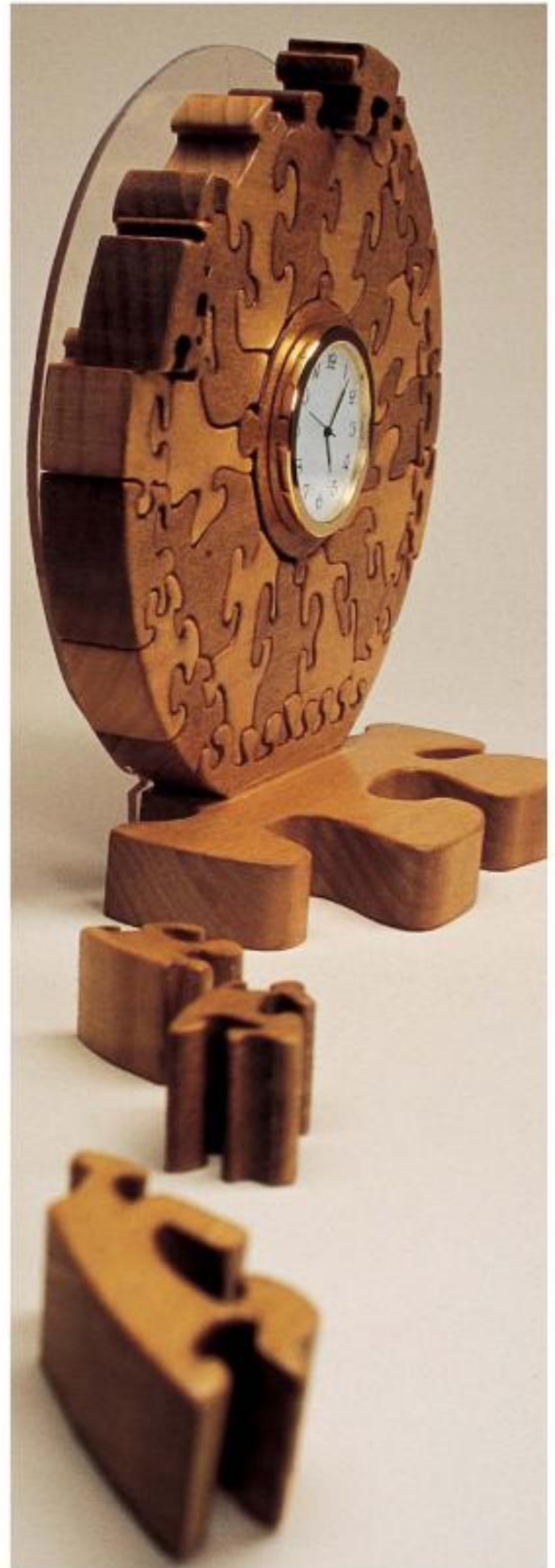
Anatomy of a puzzle clock: A \frac{1}{16} " Plexiglas backing board serves as the backbone of this curious puzzle clock. The backer was scrolled with a #2 skip-tooth blade. This clock features a 2" movement housed in a 1\frac{13}{16} " hole, which is \frac{1}{4} " deep.
