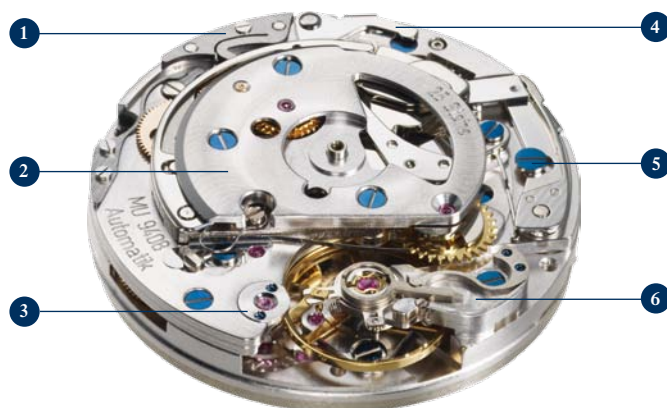
Functional and aesthetic finishes at Mühle-Glashütte: 1) straight graining, 2) Glashütte solarization, 3) circular graining, 4) polishing, 5) blued screws, 6) perlage.
