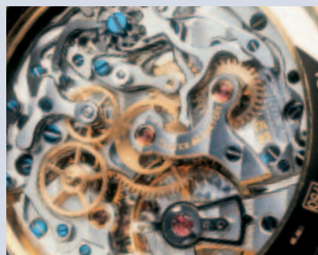
ML 83/72 movement based on Valjoux 23/72C.
