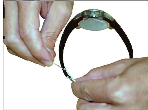
Step 3A: Use a push device, such as a small paper clip on the 6 o'clock side of the watch, and insert it into the hole where the spring bar sits connecting the strap and the buckle. It is important to remove the initial selections(s) from the strap section on the 6:00 side of the watch.
