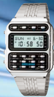
World's first databank-equipped watch, Databank Telememo 10 CD-40 1984
