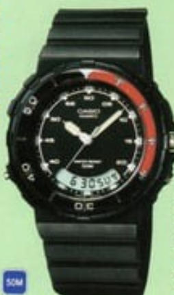
AW-32/1V Module No. 388 ○50m water resistant ○Daily alarm ○Hourly time signals ○Dual time ○1/100 sec. stopwatch Measuring range: 59:59.99" ○12/24 hour formats ○Battery: approx. 2 years on SR920W
