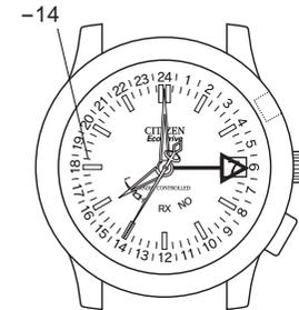
3. After setting the time, return the crown to its normal position; the second hand will move normally, and the 24-hour hand will display the set time.
