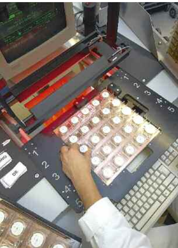
Movements arrive at COSC in clear plastic capsules with simple white dials.
