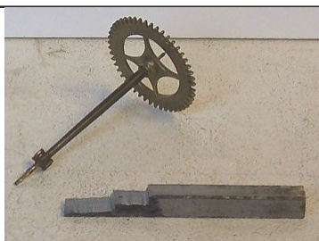
2 The hole has been drilled and the waste removed.
