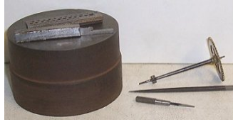
4 The drift with its holder and a steel stake with various holes. Note the drift looks larger than it should due to the camera angle.
