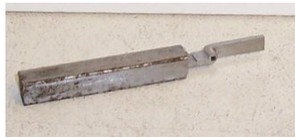
6 The pallet ready to be parted from the parent metal.
