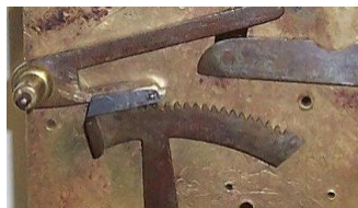
7 The rough pallet at the locked position, ready for filing and polishing.
