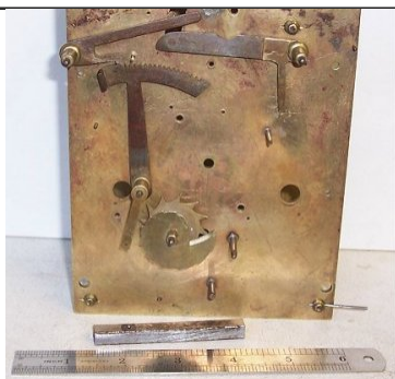
Scrap steel centre punched and ready to drill, 1-1mm.
