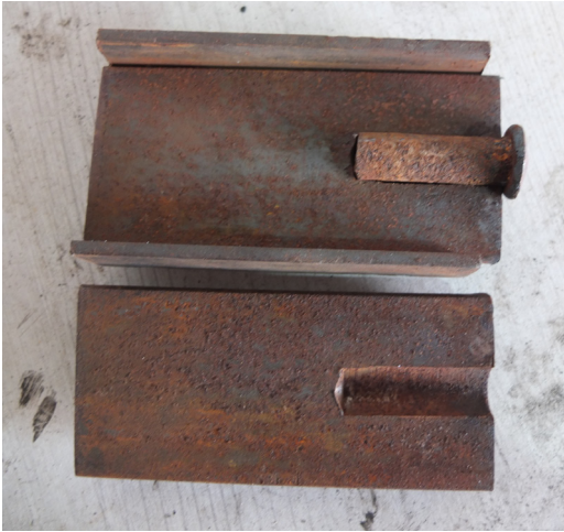
Fig. 20. A former for making rivets.
