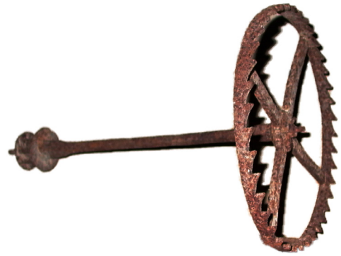
Fig. 22. A verge crown wheel escapement and pinion found nearby the clock.
