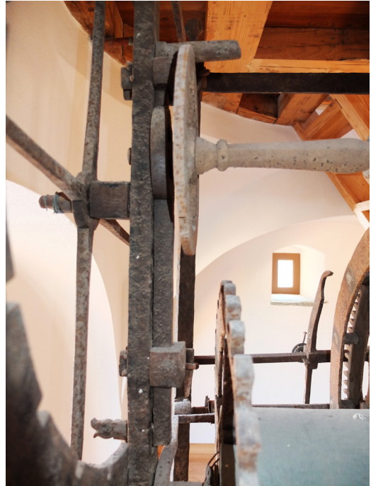
Fig. 29. The Ivron clock with the Z dual detent locking system, internal count wheel and over-lift cam wheel.
