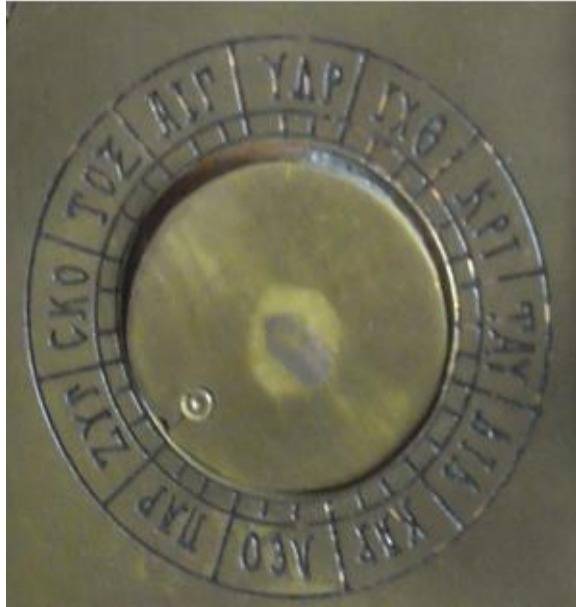
Fig 7: Byzantine sundial-calendar, detail of back face showing the Solar display (reconstruction and photo courtesy by Dionyssios Kriaris)
