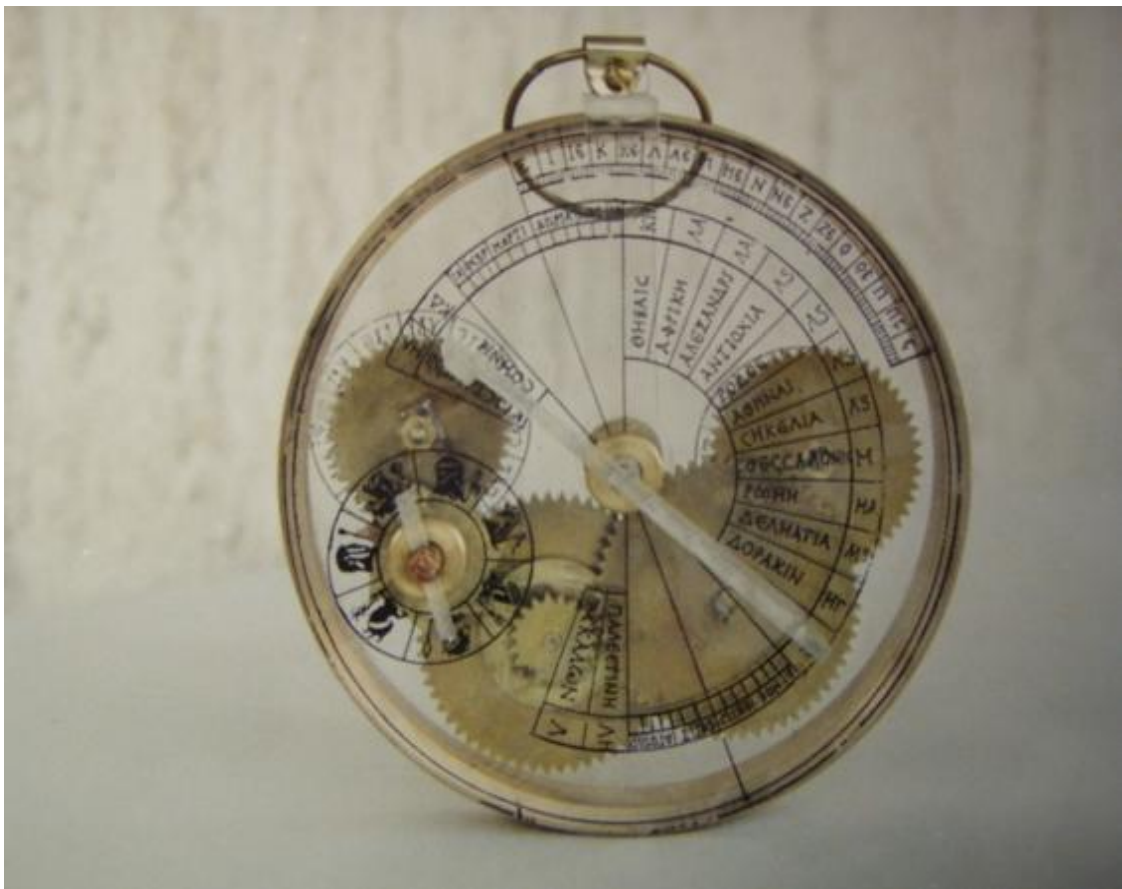
Fig. 14: Byzantine sundial-calendar, front face of transparent model showing the gear device of the instrument (reconstruction and photo courtesy by Dionyssios Kriaris).
