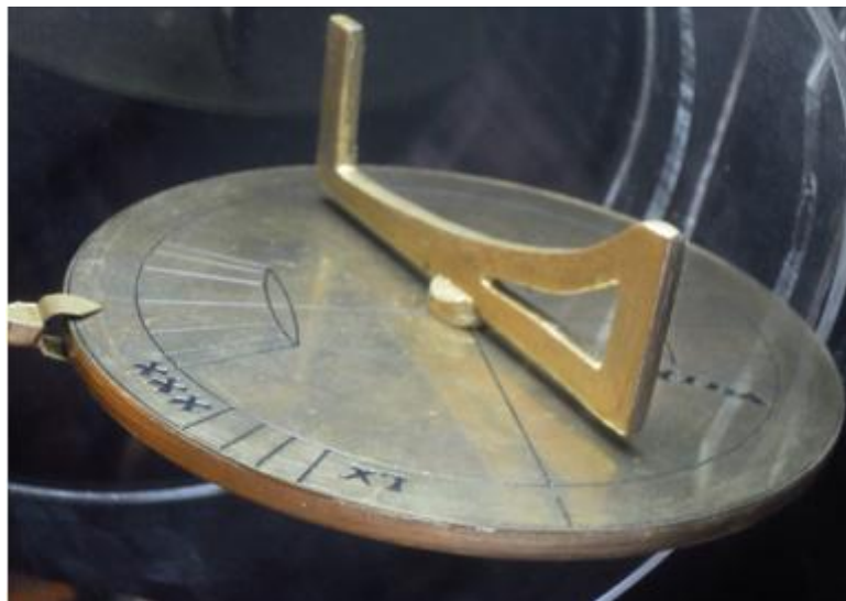
Fig 22: The Roman portable Sundial in vertical view in vertical view showing the shape of the vane with gnomon and other similar characteristics of the dial plate to the Byzantine Sundial-Calendar (reconstruction and photo courtesy by Dionyssios Kriaris).
