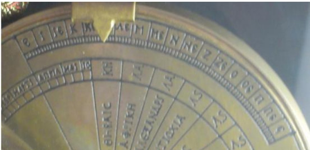
Fig 4: Byzantine Sundial-calendar, detail of front face, showing the outer scale given in degrees of latitude, with upper scale for 5^{\circ} , and inner scale for 1^{\circ} , given in greek numerals. The pointer of the arm of the instrument is set to the degree of the corresponding latitude of the user (reconstruction and photo courtesy by Dionyssios Kriaris).
