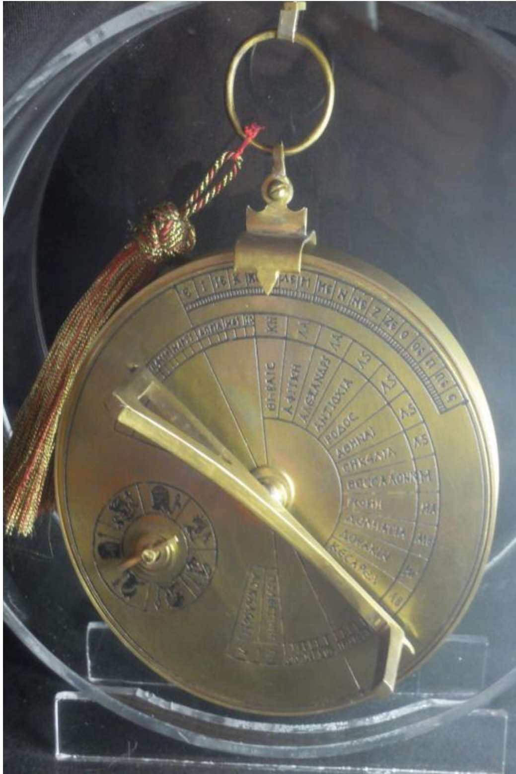
Fig. 2: Byzantine sundial-calendar, front face, (reconstruction and photo courtesy by Dionyssios Kriaris).
