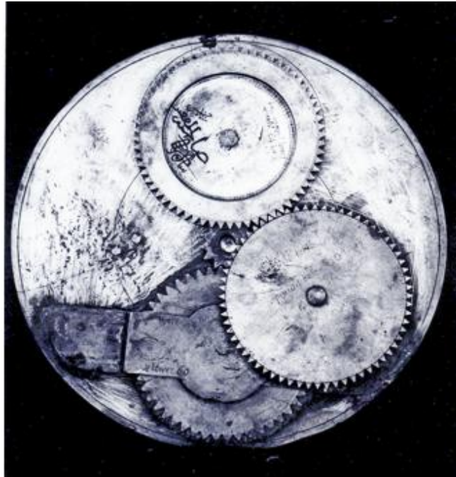
Fig. 29: Calendrical gearing in the Astrolabe-Calendar of Muhammad b. Abi-Bakr of Isfahan [by Field & Wight, 1985b].
