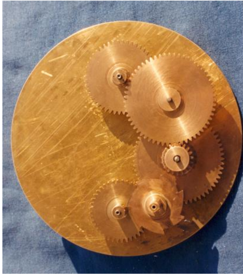
Fig. 17: Byzantine Sundial-Calendar, model of the gear mechanism, in 2:1 scale model size (reconstruction and photo courtesy by Dionyssios Kriaris).
