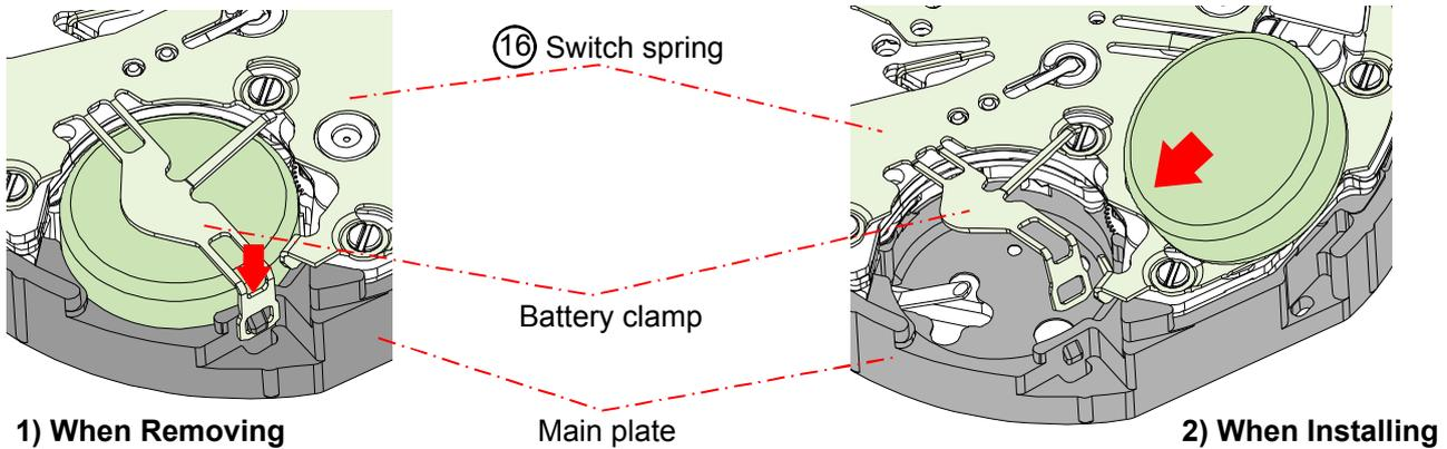
**7.Remarks on installing the battery**
