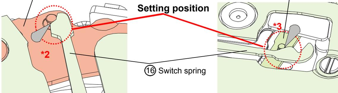
\*Oiling should be done on the contact spot of the spring and the pin.
