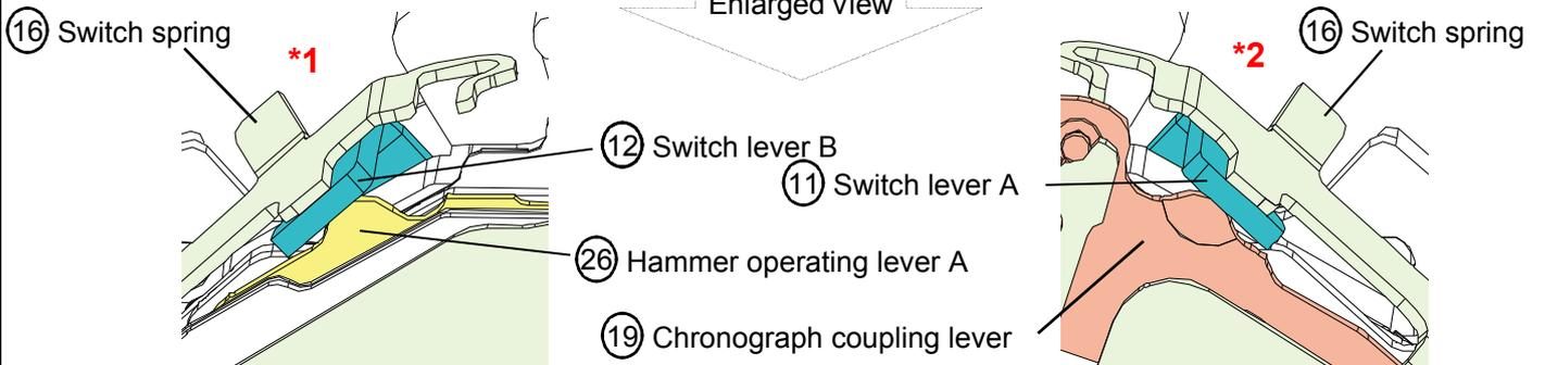
Switch lever B is set between the switch spring and hammer operating lever A
