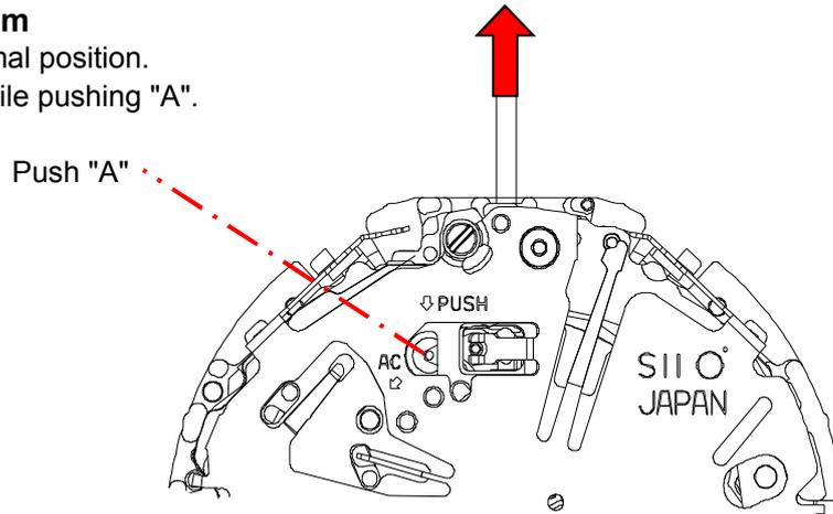
**6.To remove or install the battery**
