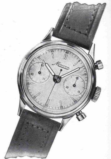
Ref. 441601 Dial 5-60 ( \frac{1}{5} -second). Case size 51 mm. 1 turn = 1 minute ; register : 60 min. with red 45 minutes sector. Functions : Start - Stop - Start by crown pressure. Fly-back to zero by depression of the lateral push-piece, the stopwatch being first stopped.
