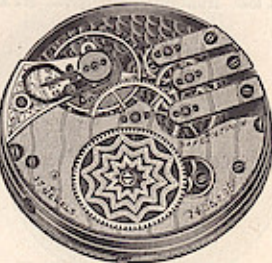
Springfield, Illinois, Movement. Nickel, 17 red jewels, composition settings, compensation balance, timing screws, finely finished beveled train, polished center wheel, counterpoised fork and pallet, best quality Swiss Breguet hairspring, Philippe coil, patent micrometric screw regulator, visible winding wheel, Swiss mainspring, double sunk dial, handsomely damasked. A thoroughly finished watch throughout. No. 1079 Hunting style ..... $26 70 No. 1080 Open Face style ..... $6 70
