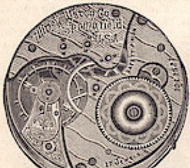
Springfield, Illinois, Movement. Nickel, 17 red jewels, composition settings, compensation balance with timing screws, counterpoised fork and pallet, highly polished beveled center wheel, best quality Swiss Breguet hairspring, Philippe coil, patent micrometric screw regulator, concave visible winding wheel, Swiss mainspring, double sunk dial, handsomely damasked, gold lettering. An attractive and well finished watch throughout. No. 1075 Hunting style ..... $24 70 No. 1076 Open Face style ..... $4 70
