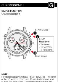
For all chronograph functions- RESET TO ZERO - The hands of the 60 seconds chrono and 30 minutes timers are reset to zero. The hand of the 1/10 second timer indicates the alarm status.
