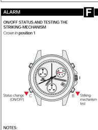
NOTES: The alarm device is alternately activated (ON) or deactivated (OFF).
