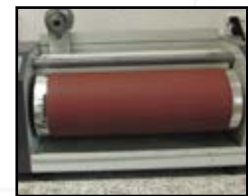
Cylindrical Drum Abrasion Resistance (ISO 4649)
