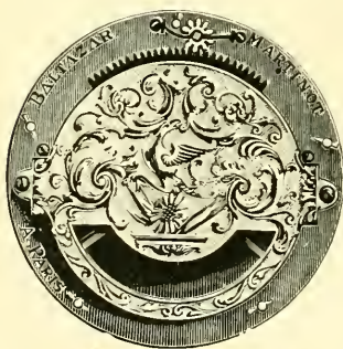
FIG. 696.—Watch by Baltazar Martinot, showing early French arrangement of balance spring regulator.
