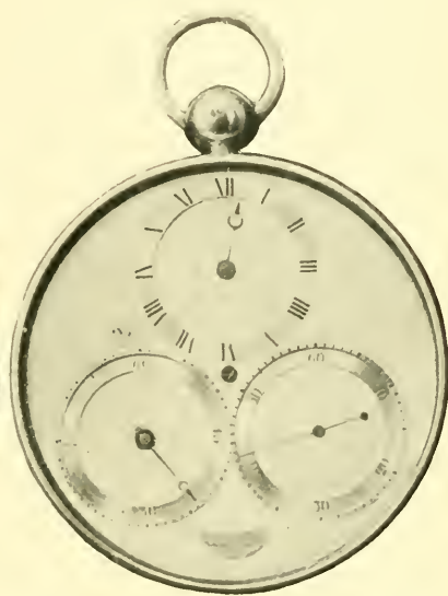
FIG. 481. Watch with chronometer escapement mounted in tourbillon carriage.
