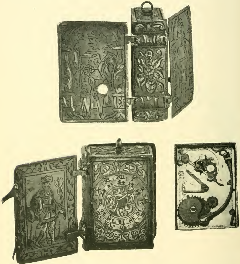
FIGS. 149—151.—Sixteenth century book-watch. Outside with covers open, inside of front cover and dial. View of mechanism inside back cover.
