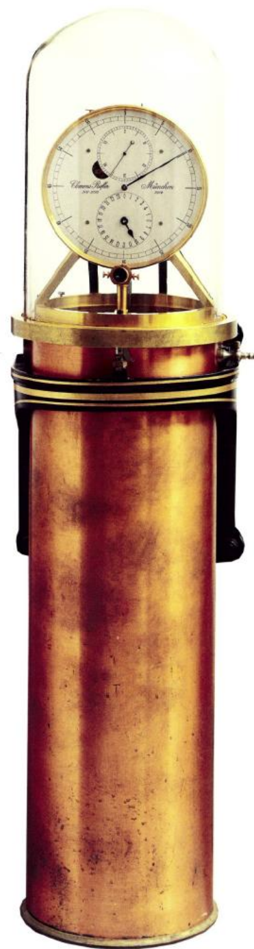
Several reference clocks kept time in the time-service room and atop granite foundations in the cellar of the German Naval Observatory. One such timepiece was this precise clock: No. 223, made by Clemens Riefler in Munich
