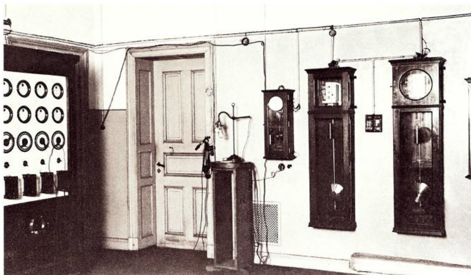
One-second pendulum clocks at the German Naval Observatory in Hamburg kept reference time for all nautical and aeronautical events
