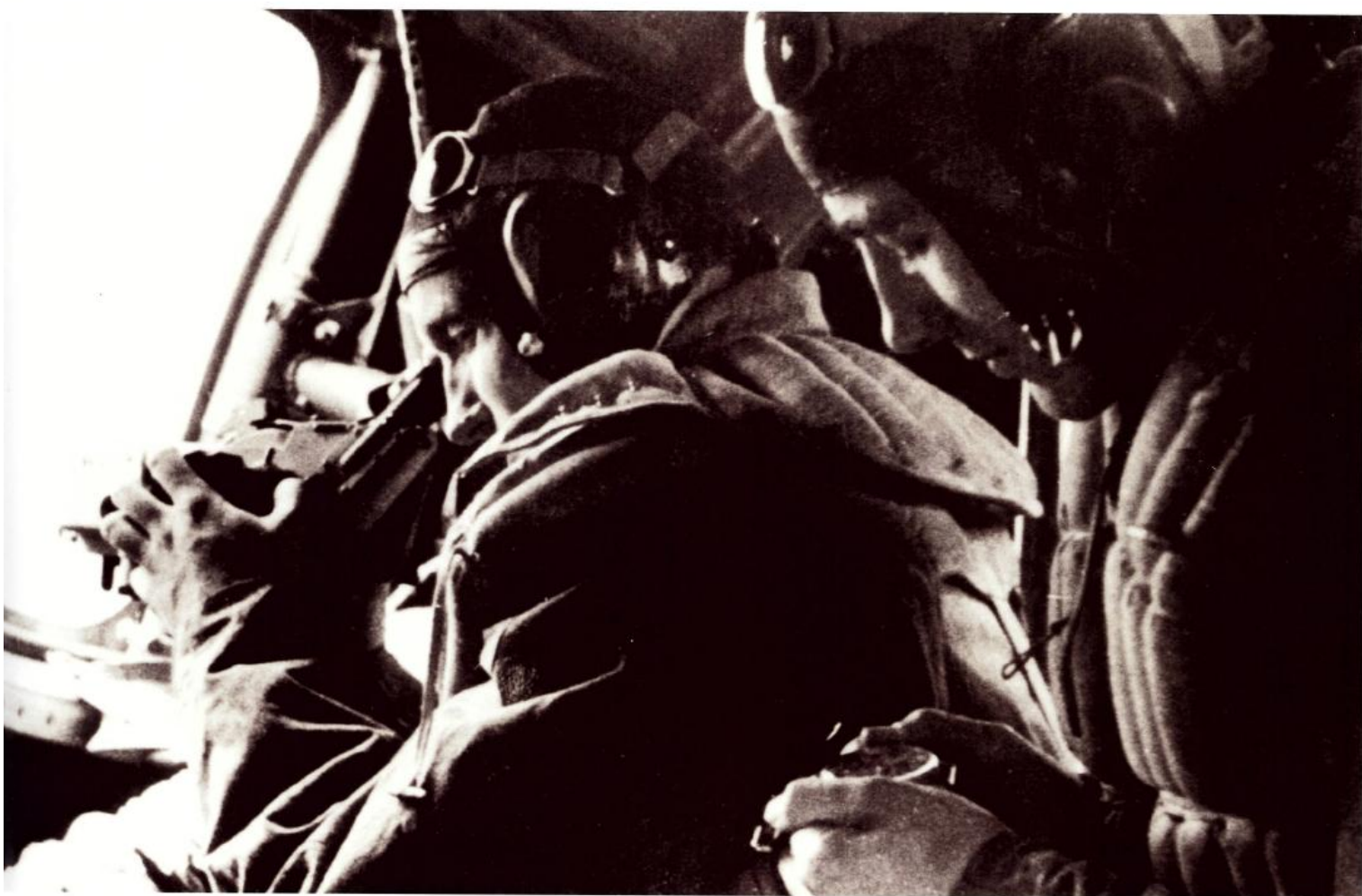
The dragonfly octant and the deck watch were used to determine an aircraft's momentary position during a long-haul flight
