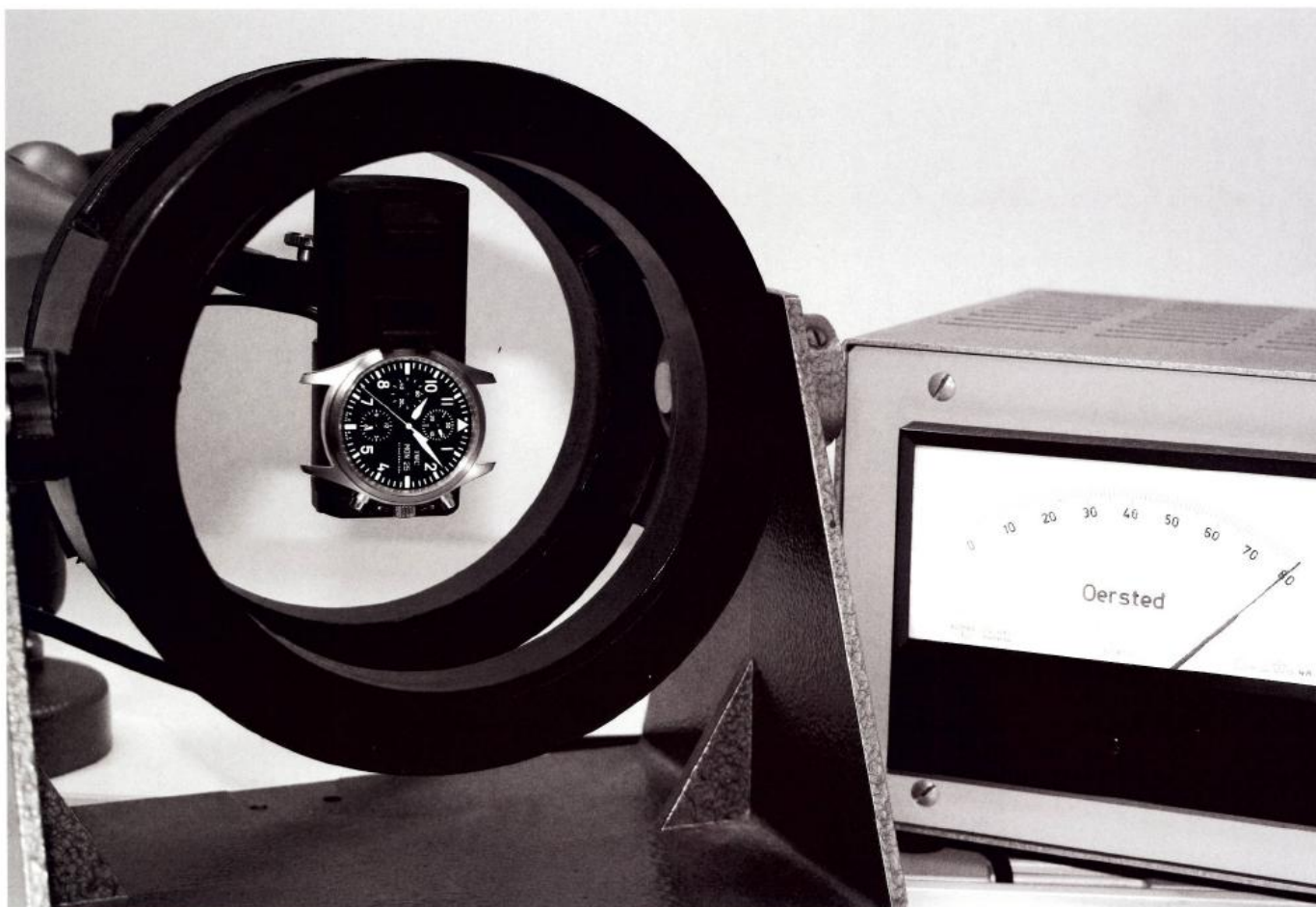
The self-winding pilot's chronograph undergoes a magnetic-field test
