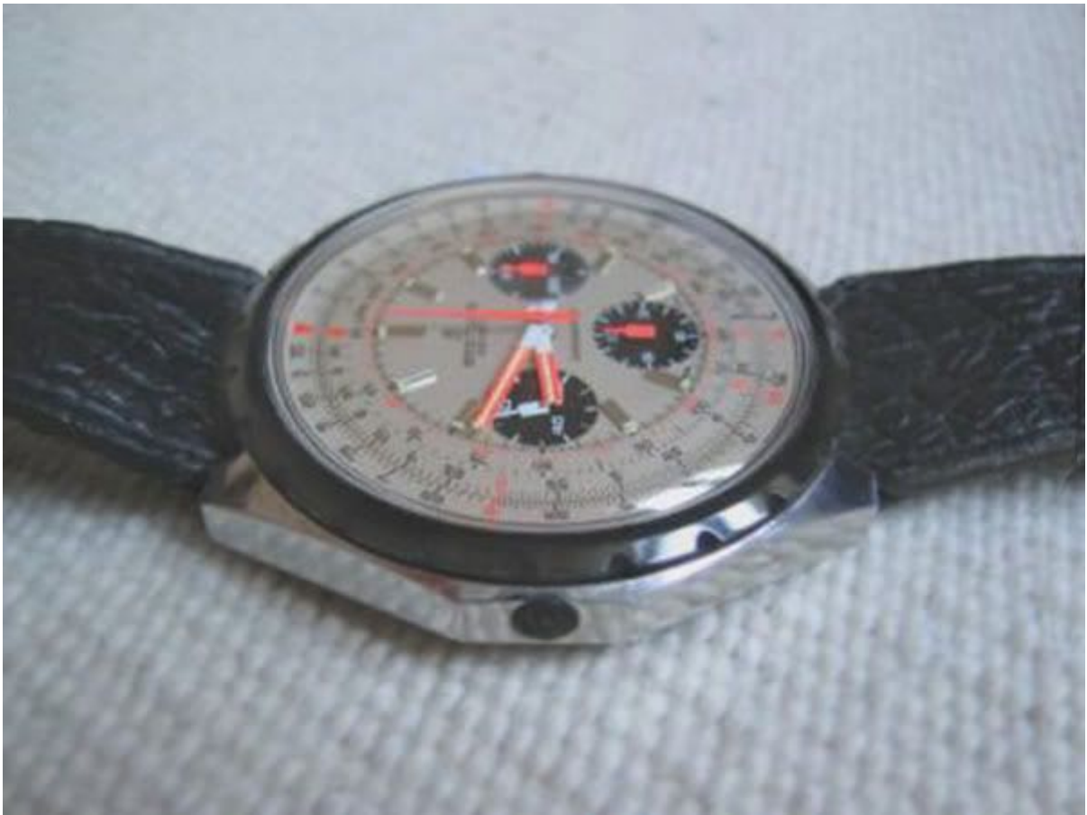
The ref 818 bezel inspection/servicing plug is in the side of the case
