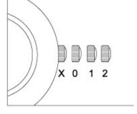
X = normal position0 = winding position1 = date adjustment
