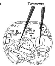
2) When the battery replaced with a new one, the time information stored in the built-in IC and the time indicated by the stopwatch hands do not correspond with each other. Reset the stopwatch hands to "0" position following the procedure below. If the stopwatch hands should move improperly, also follow the same procedure.
