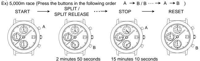
\* Measurement and release of the split time can be repeated as many times as necessary by pressing button B.
